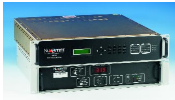
FT6 Transmitter and MM200 Multi-Rate Modem offers digital transport up to 120 Mbps (see page 8)
